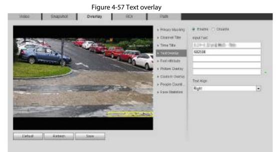
Step 2 Select the **Enable** checkbox, enter the text you need, and then select alignment. The text is
