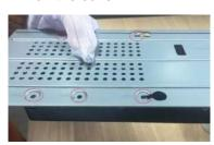
4. Match the holes on the bracket with the screw holes on HDD.
