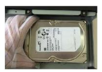
3. Put the HDD into the Device.
