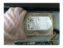
Place the HDD onto the Device.
