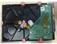
2. Fix the screws onto the HDD, but do not be fastened.
