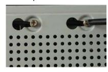
Turn the device to see the back side of it. Aim the screws of the HDD at the holes on the back of the
