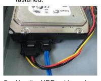
Use the HDD cable and power cable to connect HDD and mainboard.
