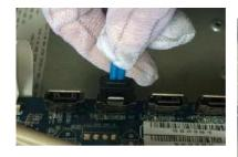
Connect the other end of HDD cable to the mainboard
