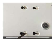
Turn the device to see the back side of it. Aim the screws of the HDD at the holes on the back of the device, and then fix the screws.
