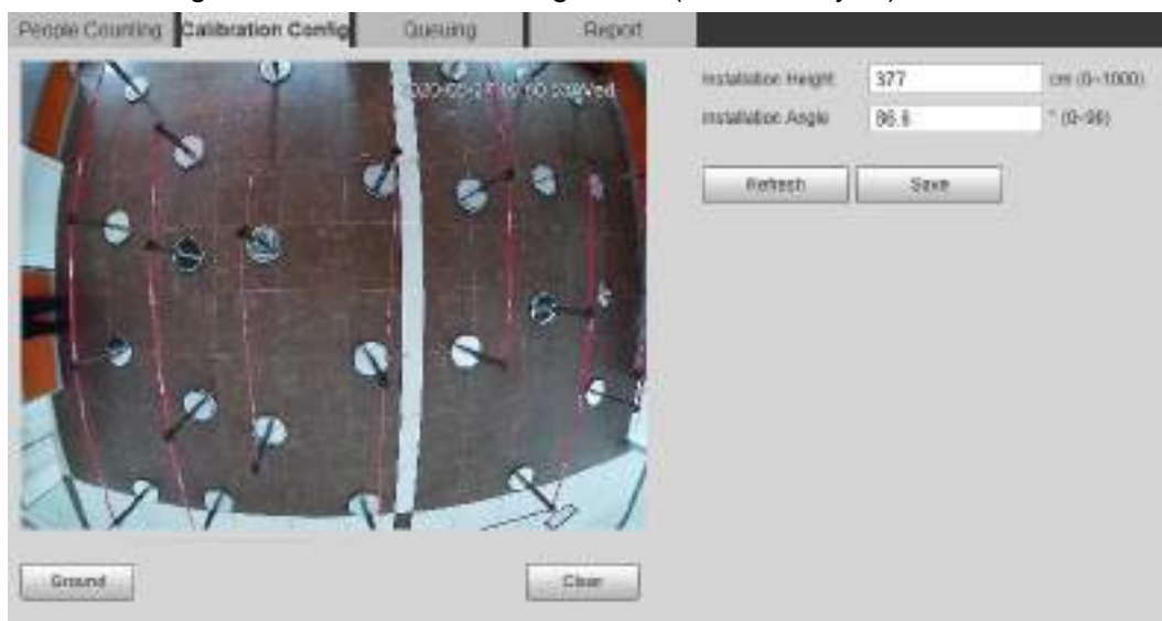
Figure 5-61 Calibration configuration (stereo analysis)
