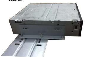
③ Fix the CD-ROM bracket at the HDD ④ Install a pair of the CD-ROM bracket. Please make sure the reverse side is secure too.
