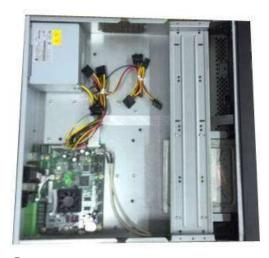
7 Put the bracket back. Please adjust the 8 Connect the SATA cable and power wire. CD-ROM to the proper position so that the button of the front panel is directly facing the pop-up button of the CD-ROM.
