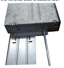
⑤ Install SATA burner. Line up the SATA burner to the hole positions.
