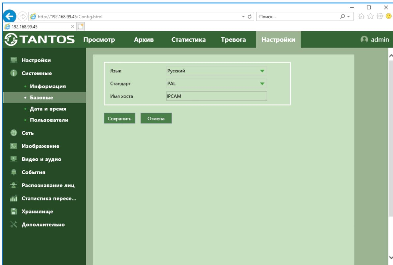
The screenshot shows the TANTOS IP camera configuration interface. The left sidebar has a dark green background with white icons and text. The 'Системные' section is expanded, showing 'Базовые' selected. The main panel is light green and contains three input fields: 'Язык' (Language) set to 'Русский', 'Стандарт' (Standard) set to 'PAL', and 'Имя хоста' (Host Name) set to 'IPCAM'. Below these fields are two buttons: 'Сохранить' (Save) and 'Отмена' (Cancel).
