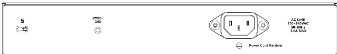
Figure 2-10 – DGS-1100-26 Rear Panel
