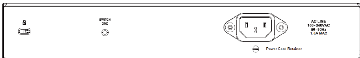
Figure 2-4 – DGS-1100-18 Rear Panel
