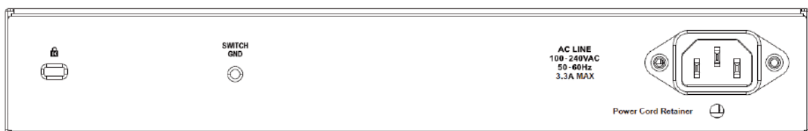
Figure 2-8 – DGS-1100-24P Rear Panel
