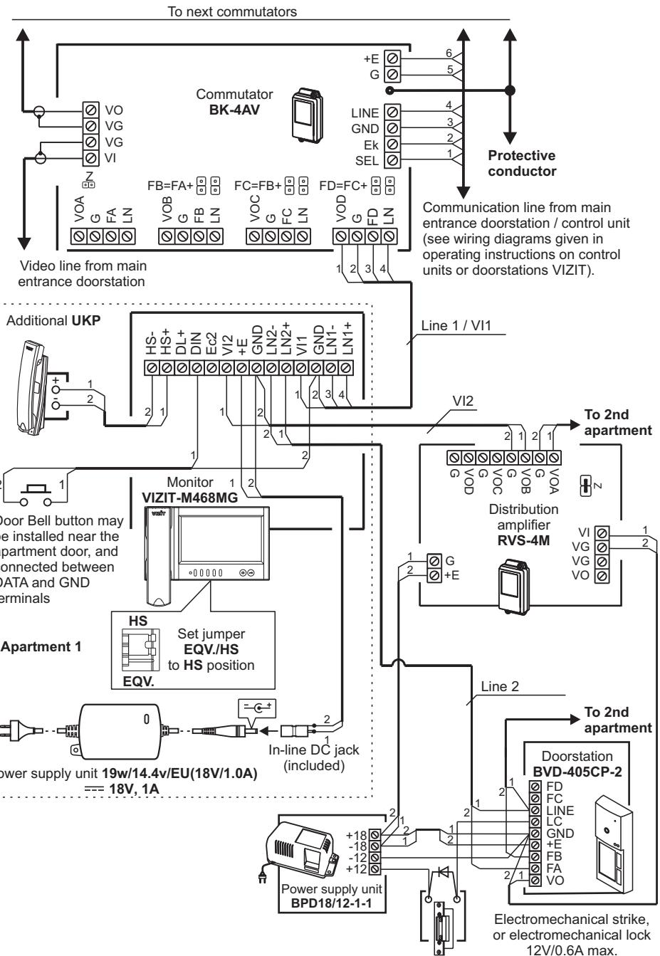
Monitor VIZIT-M468MG(MS) with commutator for multi-apartment video doorphone, 2-subscriber individual doorstation, additional apartment handset UKP, and Door Bell button.
