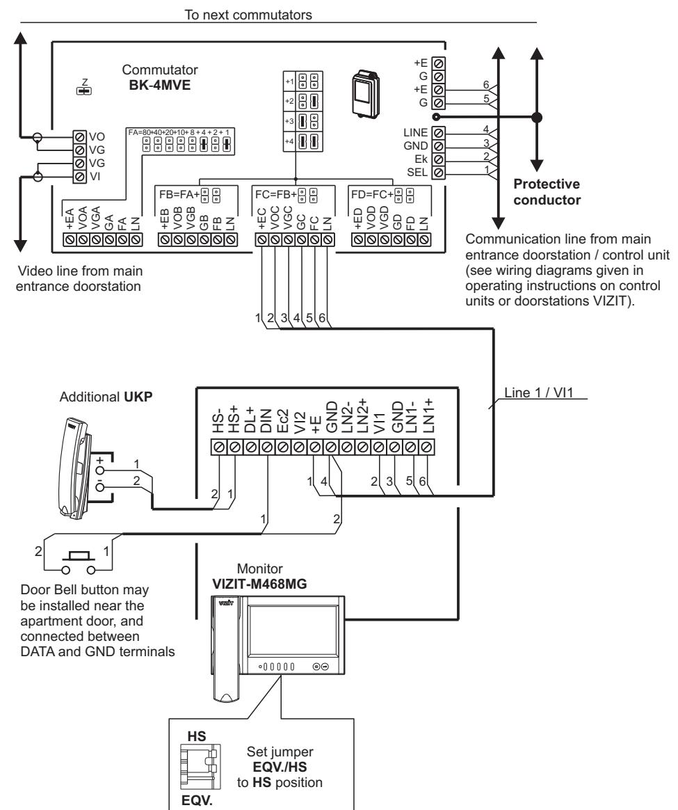
Monitor VIZIT-M468MG(MS) with commutator for multi-apartment video doorphone, additional apartment handset UKP, and Door Bell button.
