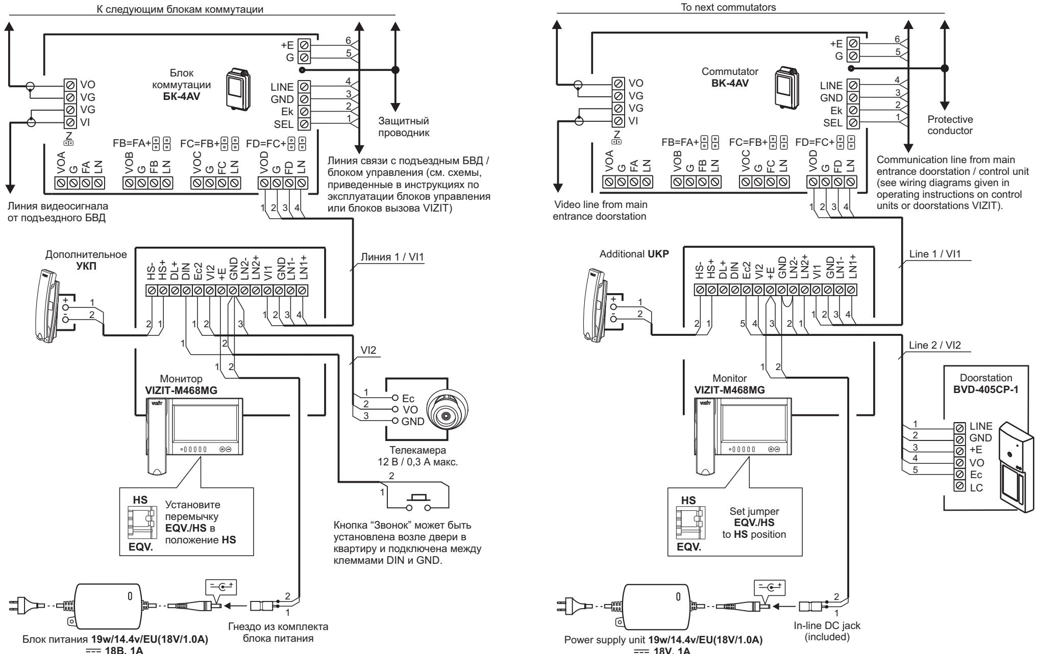
Monitor VIZIT-M468MG(MS) with commutator for multi-apartment video doorphone, 1-subscriber individual doorstation, and additional apartment handset UKP.
