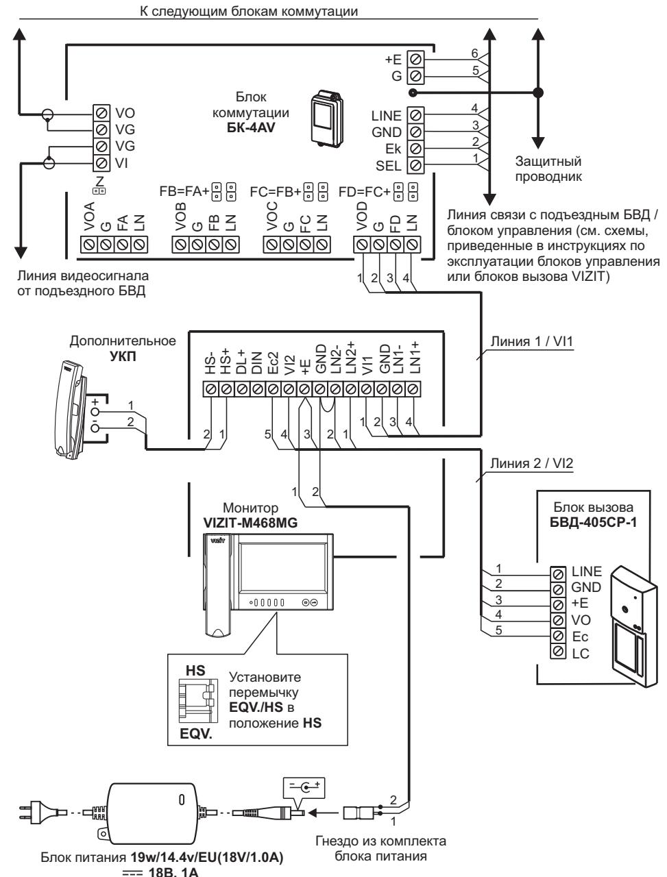
Monitor VIZIT-M468MG(MS) with commutator for multi-apartment video doorphone, additional apartment handset UKP, outdoor camera, and Door Bell button.
