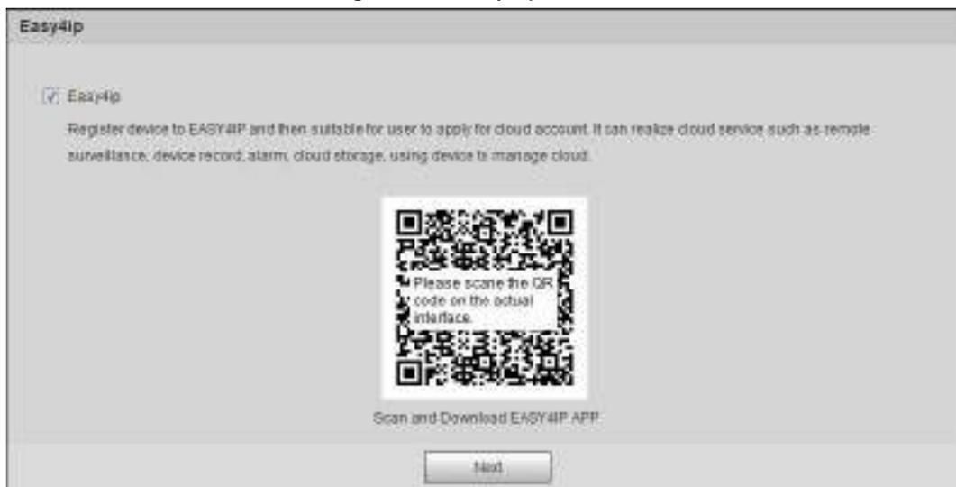
**Step 5** You can register the camera to Easy4ip, select the check box as needed, and then click **Next**.
