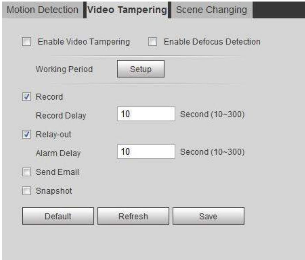
**Step 2** Select the **Enable Video Tampering** check box, and set arming periods and alarm linkage action. For details, see "5.1.1 Alarm Linkage".
