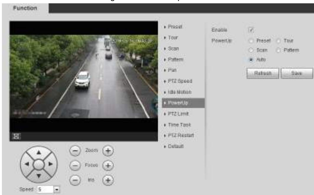
**Step 2** Select the **Enable** check box to enable the power up function.
