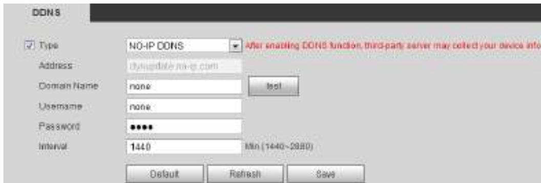
**Step 2** Select **Type**, and configure the parameters as needed.
