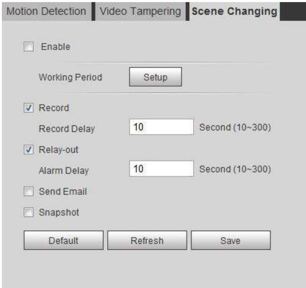
Step 2 Set arming periods and alarm linkage action. For details, see "5.1.1 Alarm Linkage".
