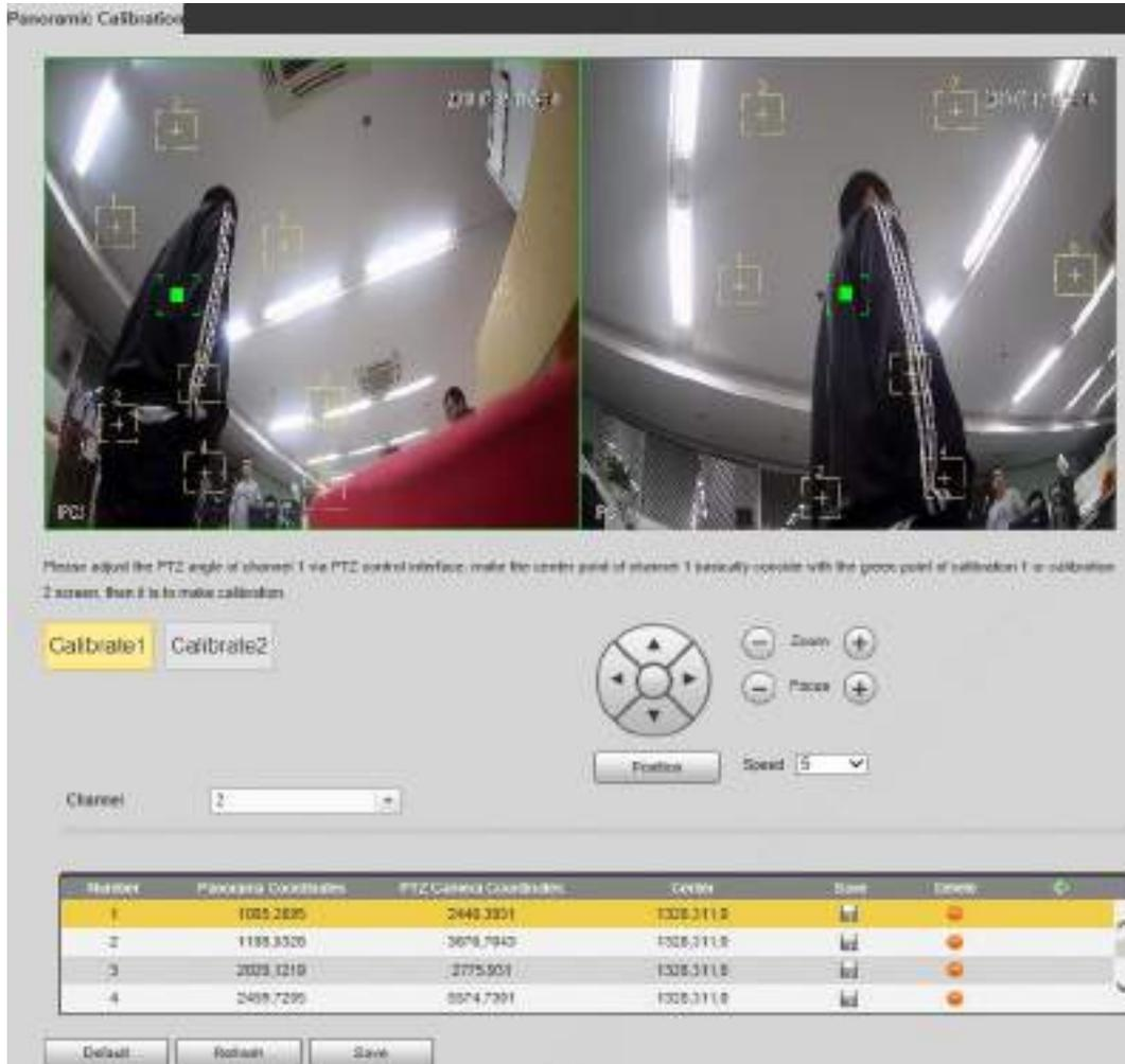
Step 2 Select channel 2, and then select a calibration number under the video images in turns (See Figure 5-20) to add calibration points to the corresponding video images. Take **Calibrate 1** as an example.
