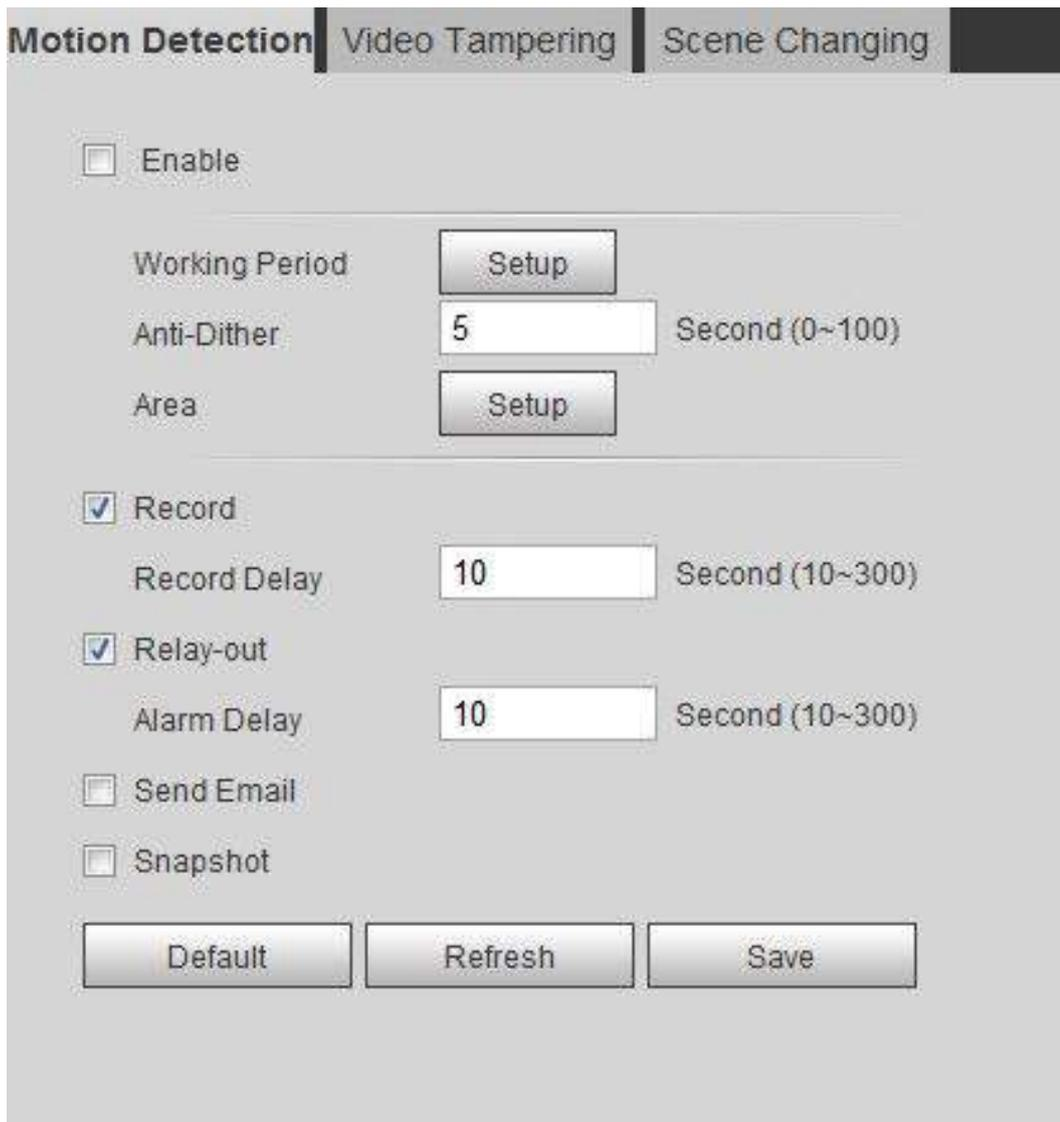
The image shows a web-based configuration interface for motion detection. At the top, there are three tabs: "Motion Detection" (selected), "Video Tampering", and "Scene Changing". Below the tabs, there are several settings:
