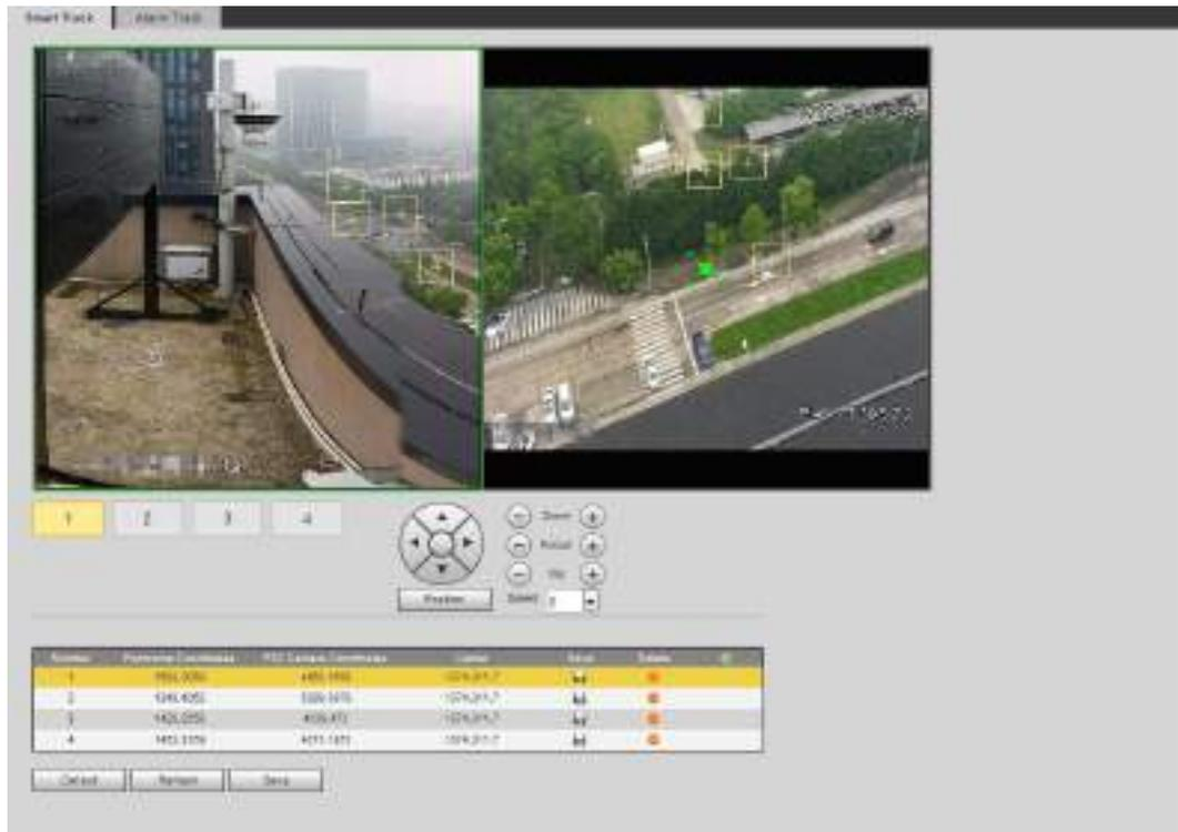
**Step 2** Select scene number under the video images in turns (See Figure 5-17) to add calibration points on the video images of the corresponding scene. Scene numbers 1 to 4 are four splitting scenes of spliced image, and at least add four calibration points on each scene.
