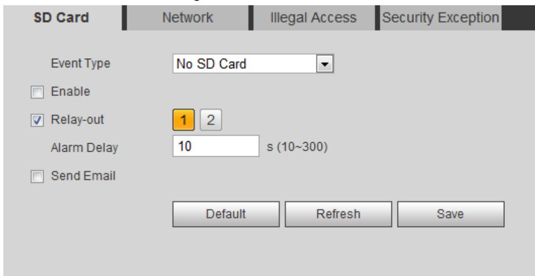
Step 2 Select the event type from the **Event Type** drop-down list, and then select the **Enable** check box to enable the SD card detection function.
