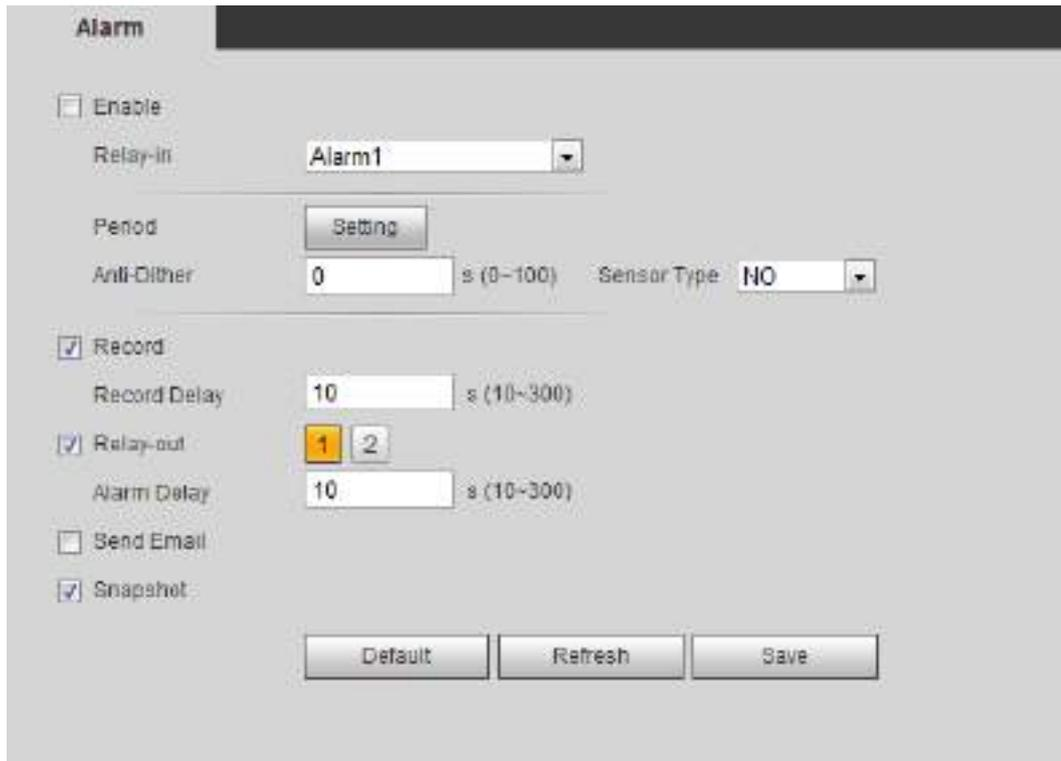
**Step 2** Select the **Enable** check box to enable the alarm linkage function.
