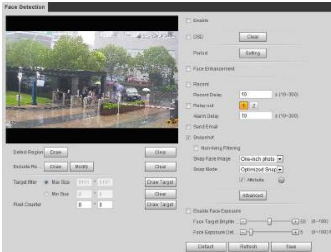
**Step 2** Select the **Enable** check box to enable the face detection function.
