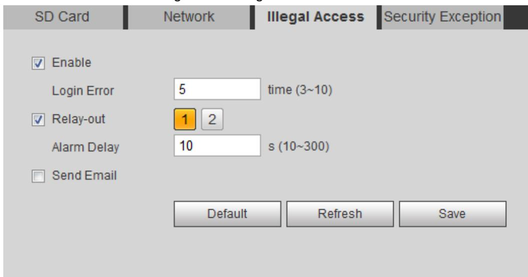
Step 2 Select the **Enable** check box to enable the illegal access detection function.
