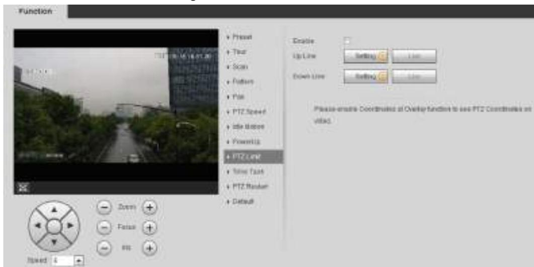
**Step 2** Adjust the direction buttons, and then click **Setting** ① to set the up line; click **Setting** ② to set the down line.
