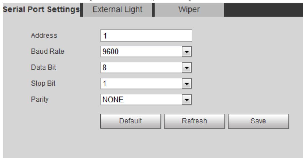
**Step 2** Configure serial port settings parameters.
