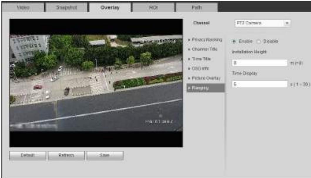
Step 2 Select the **Enable** check box, and then set the installation height and time display.
