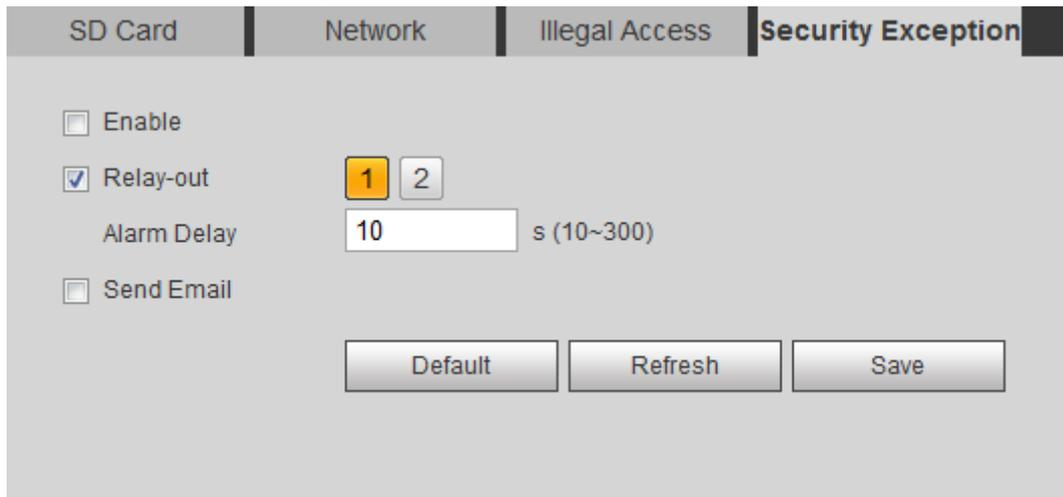
Step 2 Select the **Enable** check box to enable the security exception detection function.
