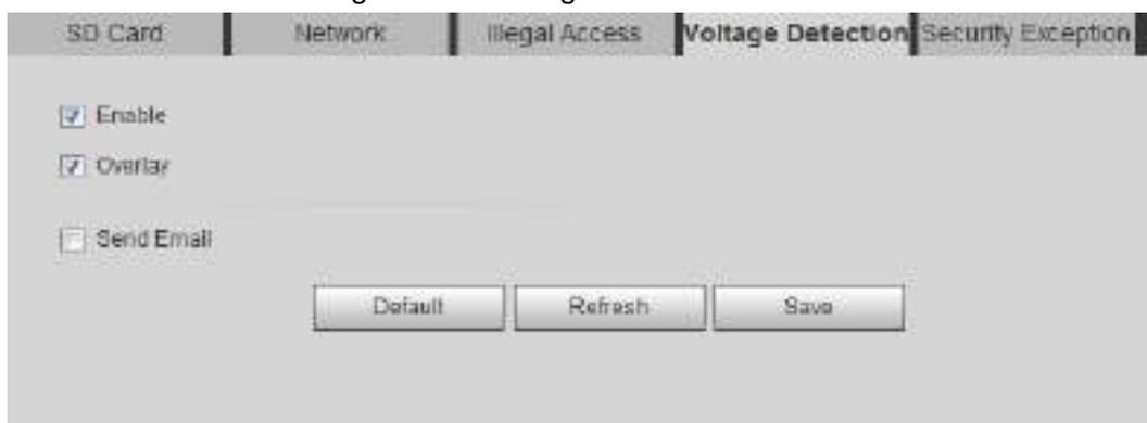
Step 2 Select the **Enable** check box to enable the voltage detection function.
