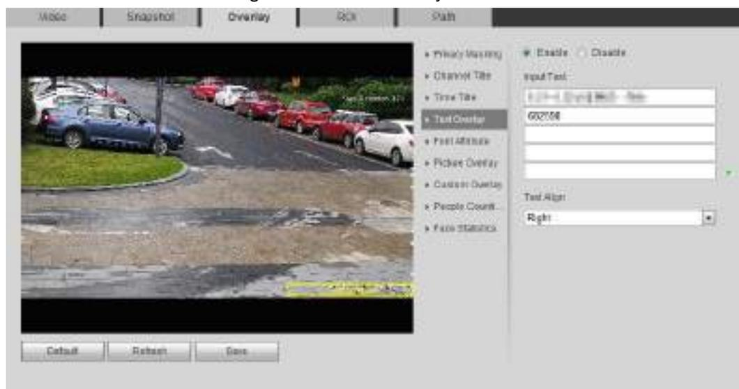
Step 2 Select the **Enable** check box, enter the text you need, and then select alignment. The text is displayed in the video image.
