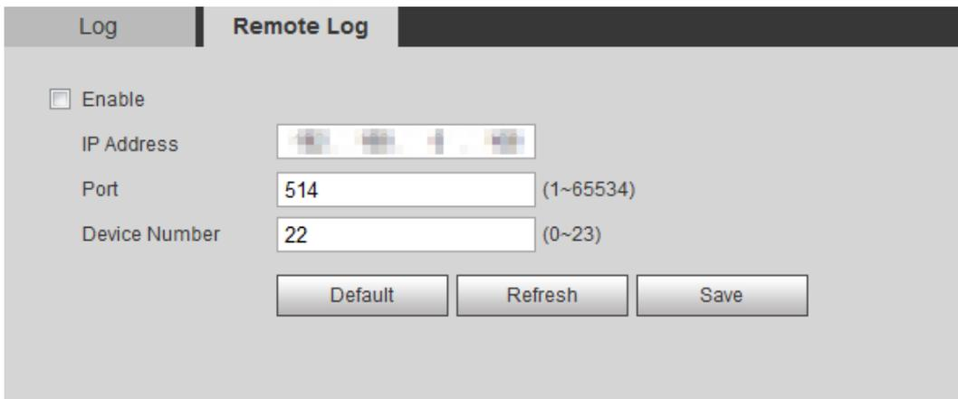
Step 2 Select the **Enable** check box to enable remote log function.
