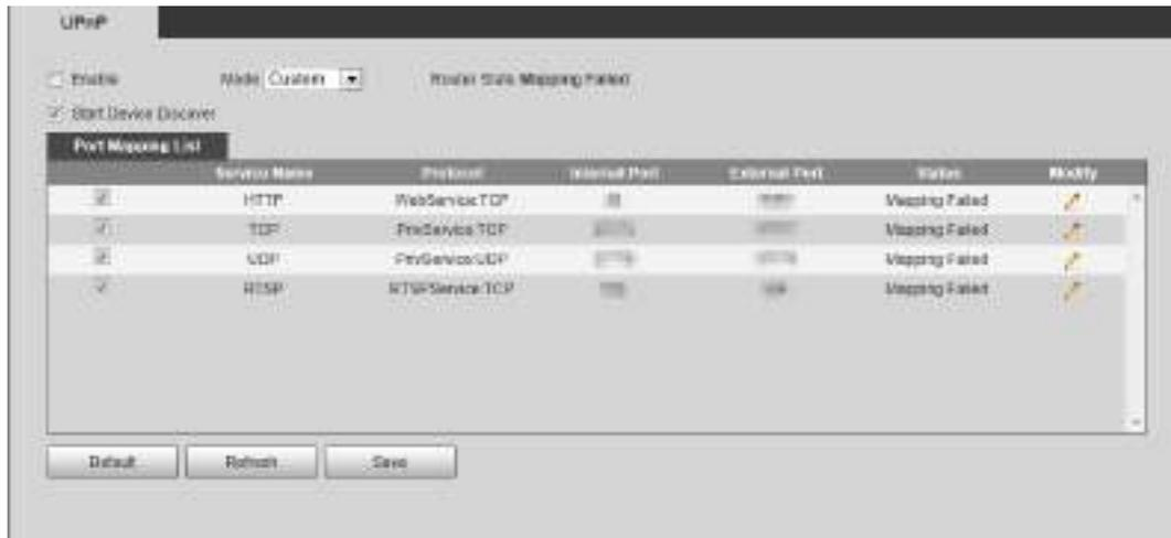
**Step 2** Select the **Enable** check box, and there are two mapping modes: **Custom** and **Default**.
