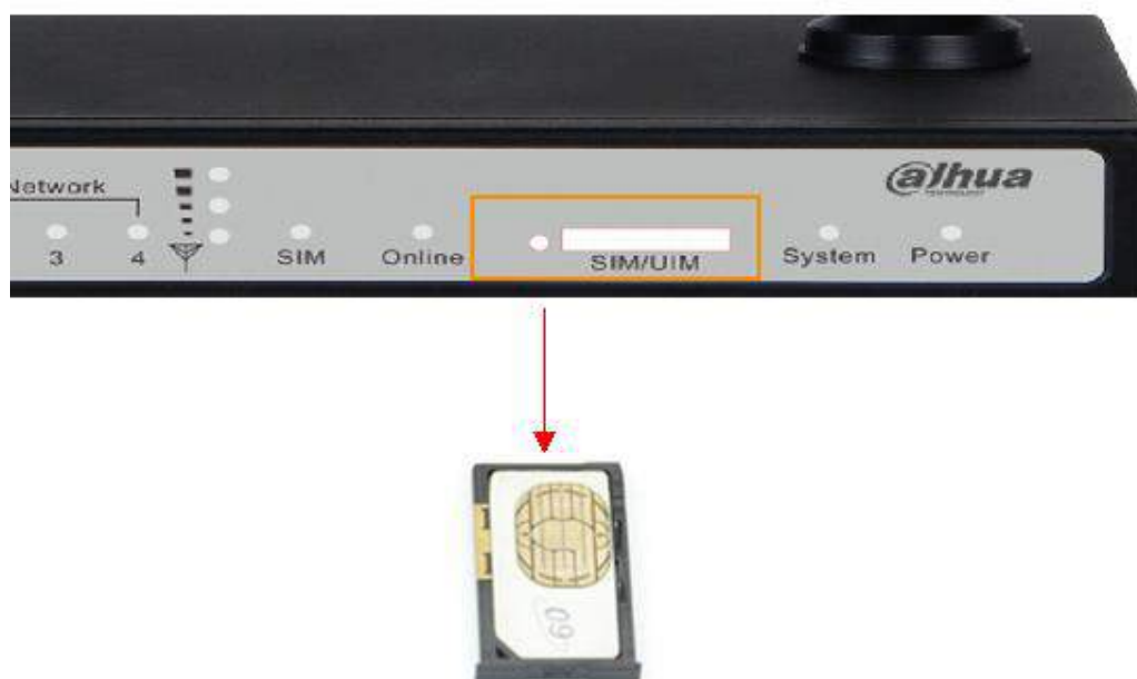
Figure 2-3 SIM/UM card installation
