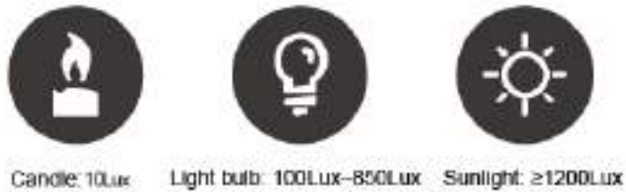
Figure 2-5 Ambient illumination requirement
