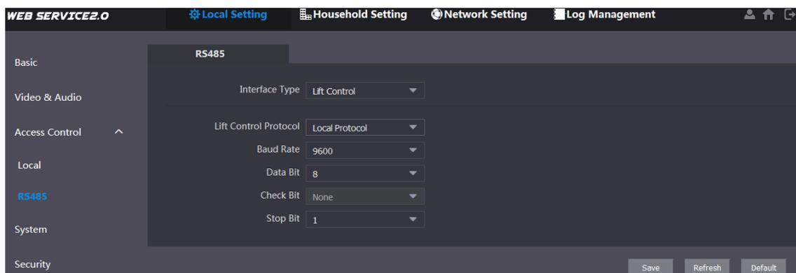
**Step 2** Configure parameters, and you can select **Lock** or **Lift Control** in the **Interface Type** list. For the detailed description, see Table 4-4.
