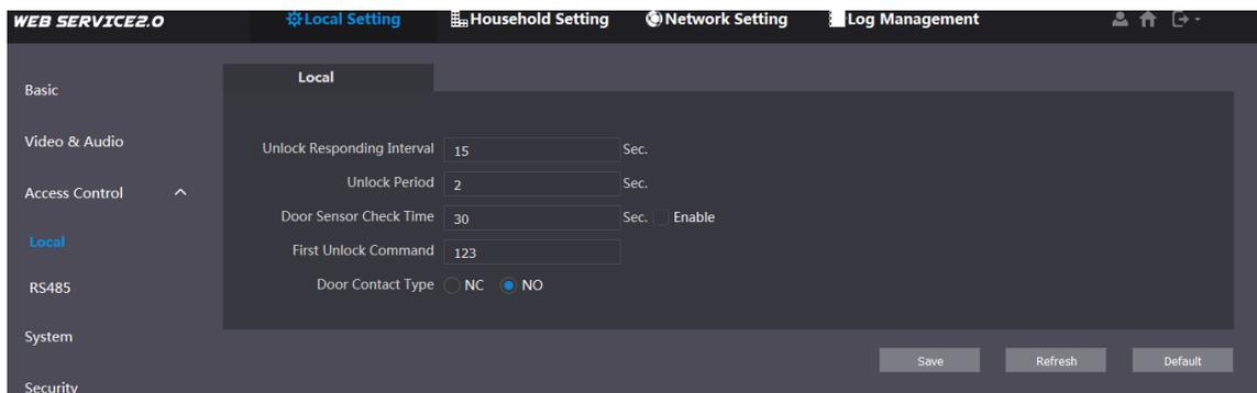
**Step 2** Configure parameters, and for the detailed description, see Table 4-3.
