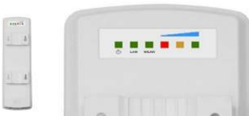
Figure 1-1 LED Indicator Light on DH-PFM881 Shell
