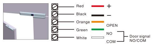
Under circumstance that two door are closed correctly by detection, lock will release signal
