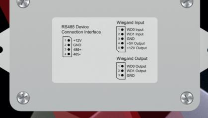
INPUT / OUTPUT EXTERNAL WIEGAND MODULE
