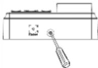
(1) Remove the screw on the bottom of device.
