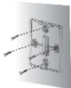
(3) Fix the back cover on the wall according to the mounting paper.
