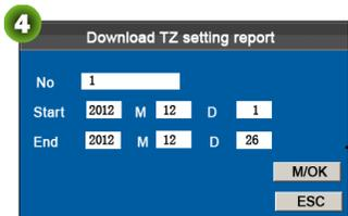
3. Enter the start and end dates then press [M/OK] key to calculating & downloading.
