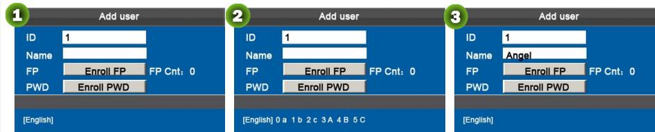
Press the [M/OK] key to enable the T9 input method.
