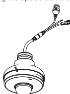
Figure 4-6 Securing the speed dome on the mounting plate
