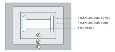
Note: Make the Receiving Coil (RX) away from the interference source. Make sure the interference level displayed on the environment inspection indicator is less than 2.
