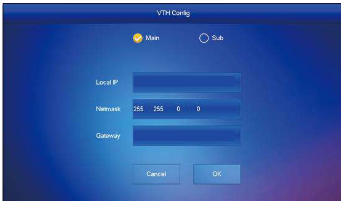
Figure 2-12 Indoor Monitor (VTH) config
