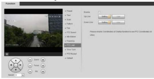
Step 2 Adjust the direction buttons, and then click Setting 1 to set the up line; click Setting2 to set the down line.
