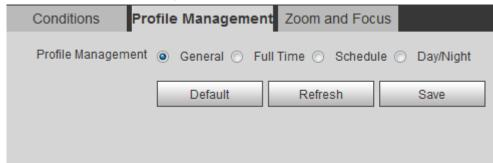
When Profile Management is set as Full Time, you can select Day or Night in the Always Enable list, the surveillance system works under Always Enable configuration.
