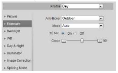
Step 2 Configure exposure parameters.
