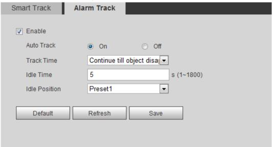
Step 2 Select the **Enable** check box to enable track linkage.
