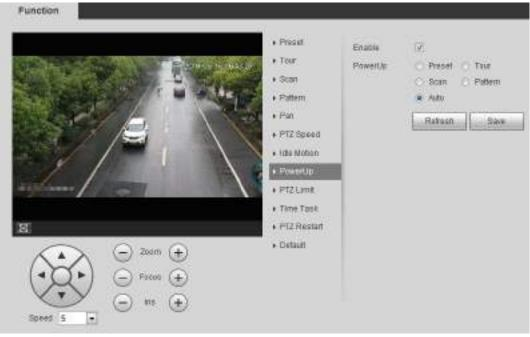
Step 2 Select the **Enable** check box to enable the power up function.
