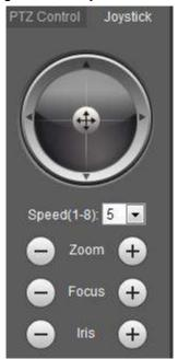
• Rotate PTZ direction through direction button. PTZ supports eight directions:
