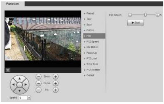
Step 2 Set the pan speed and click **Start**, and the camera starts horizontal rotation.
