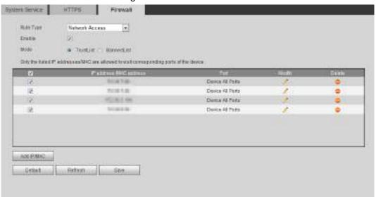
Step 2 Select **Network Access** from **Rule Type** list, and then select the **Enable** check box.
