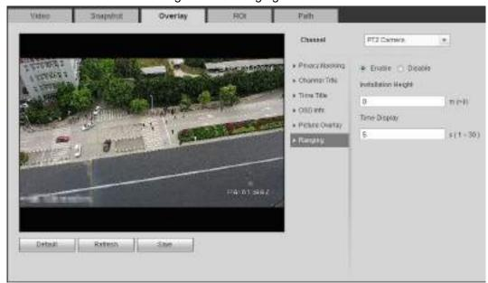
Step 2 Select the **Enable** check box, and then set the installation height and time display. Time display: The display time of the ranging information on live image.
