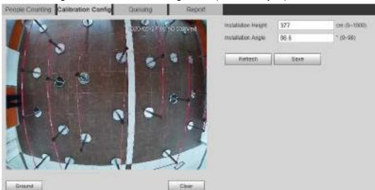
Figure 5-61 Calibration configuration (stereo analysis)
