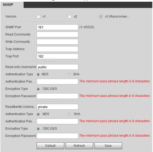
Step 2 Select SNMP version to enable SNMP.
