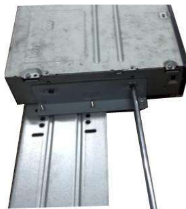
⑥ User screwdriver to fix the screws.
