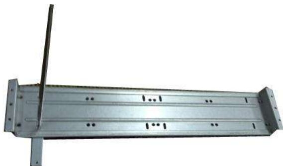
③ Fix the CD-ROM bracket at the HDD bracket.
